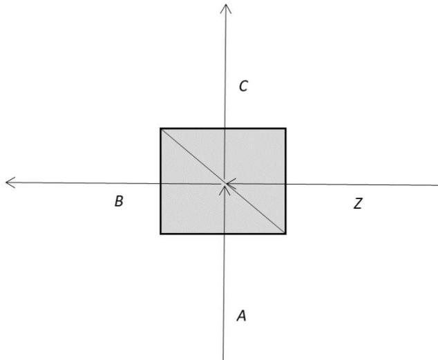
Figure 3.1: 4-port beam splitter, inputs A and Z.
