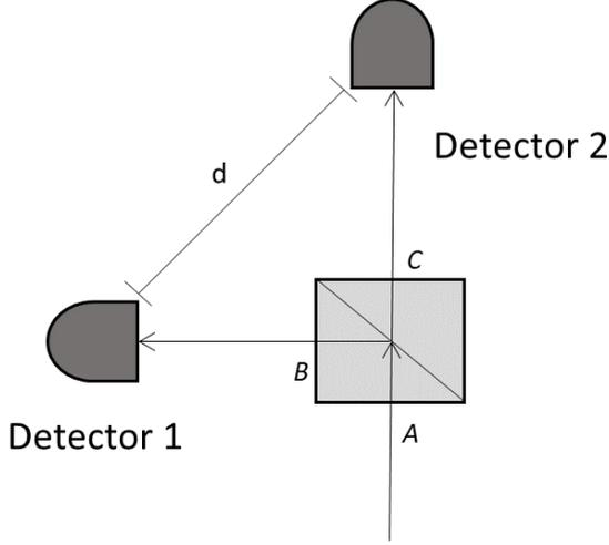
Figure 3.2: Detector configuration for a single photon impinging on beam splitter at A.
