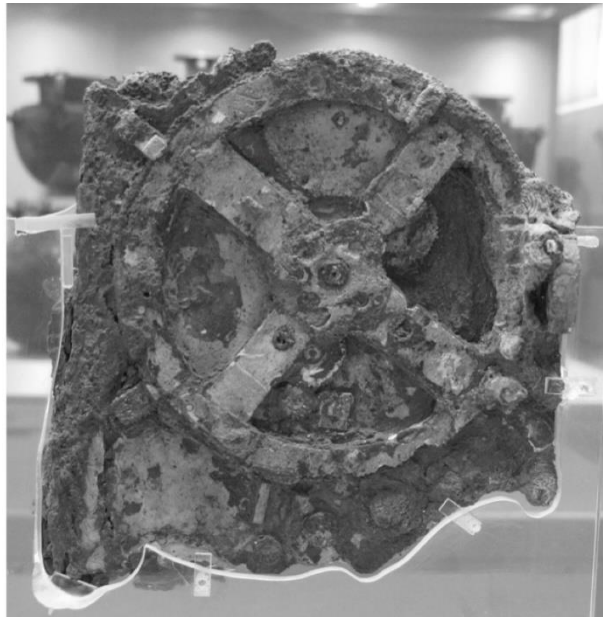
Figure 5.19: Fragment of the Antikythera Mechanism (1 BCE, Greece), an early astronomical clockwork device for computing the positions of the sun and moon.
