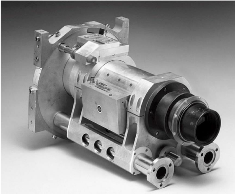
Figure 5.14: Single-photon detector, similar to that used in Hubble Space Telescope. Constructed by the Department of Physics and Astronomy, University College.
